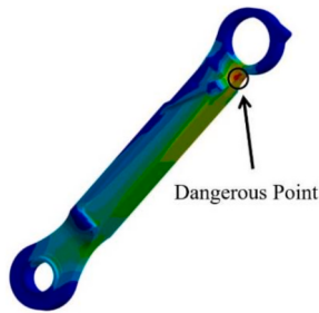
Fig. 16. Hot-spot identification from rigid-flexible simulation.
